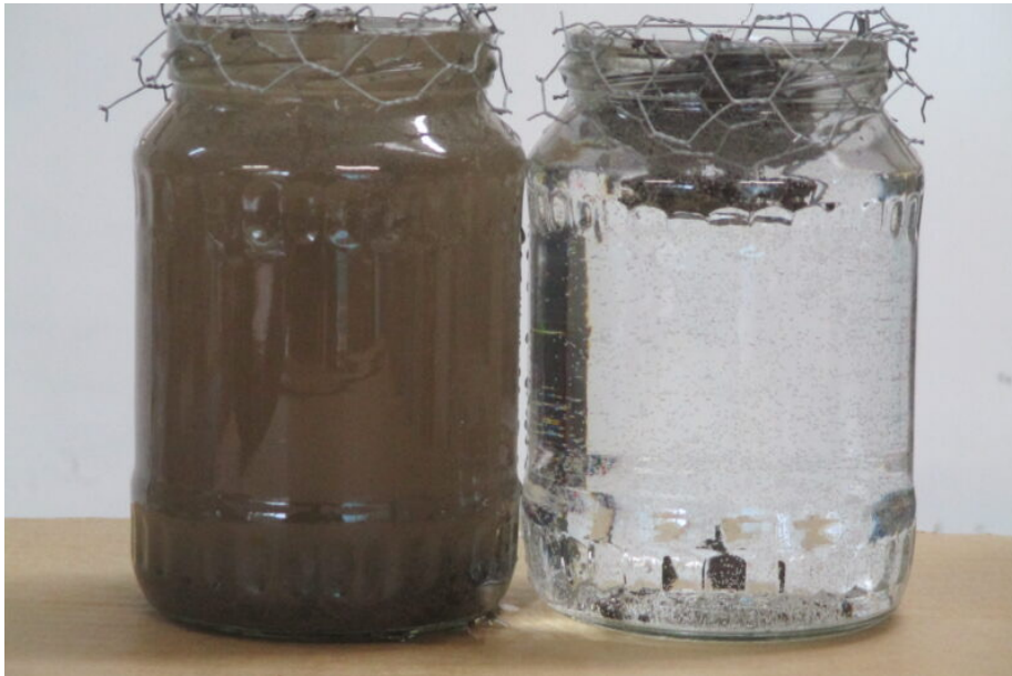
Figure 13 Slake test depicting poor aggregate stability (left) and high aggregate stability (right).
