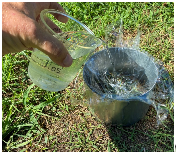
Figure 15. Adding known volume of water to the inner ring over the plastic wrap
