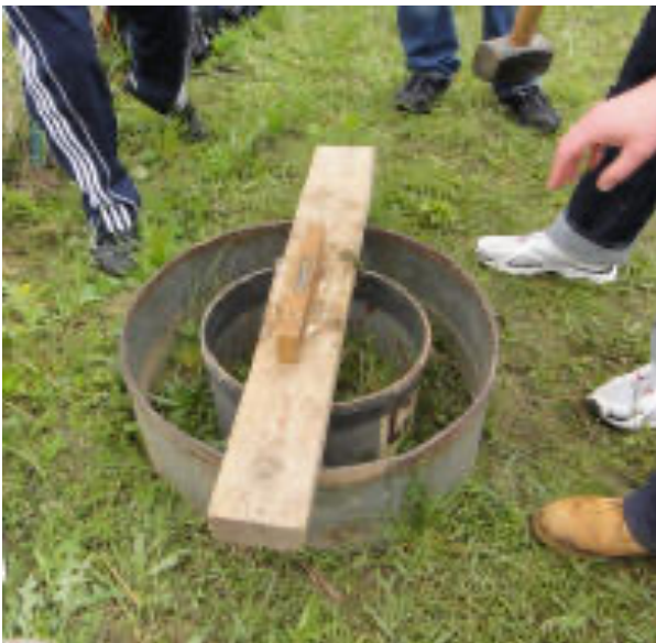
Figure 14. Driving double rings into ground.
