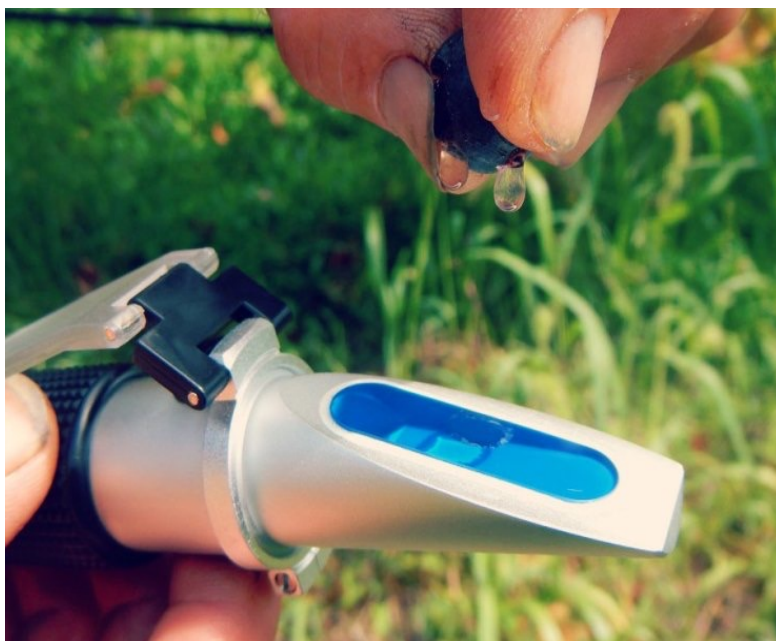
Figure 5 Squeezing plant sap onto refractometer for brix measure.
