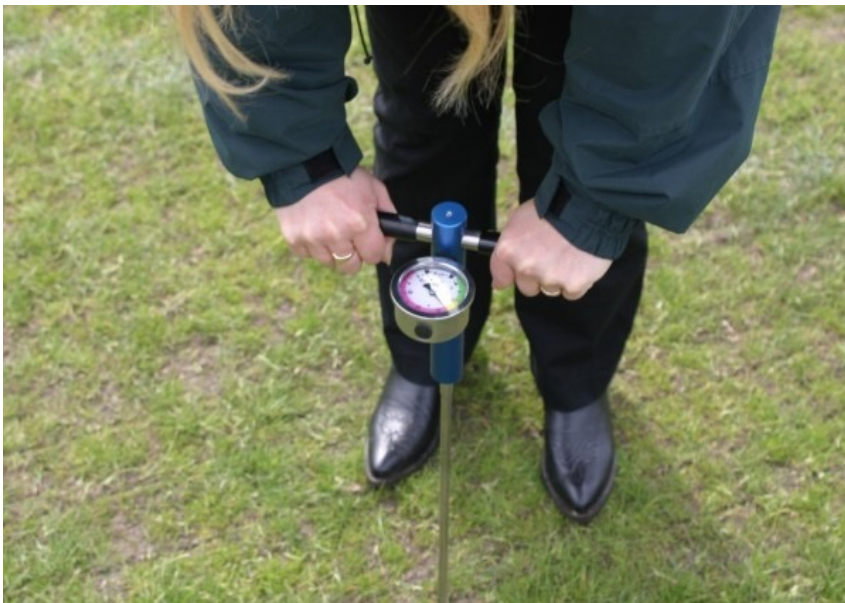
Figure 10. Measuring penetration resistance in a field using a handheld penetrometer.
