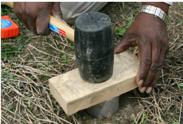
Figure 11 Driving a metal ring into the soil using a mallet and wood block.
